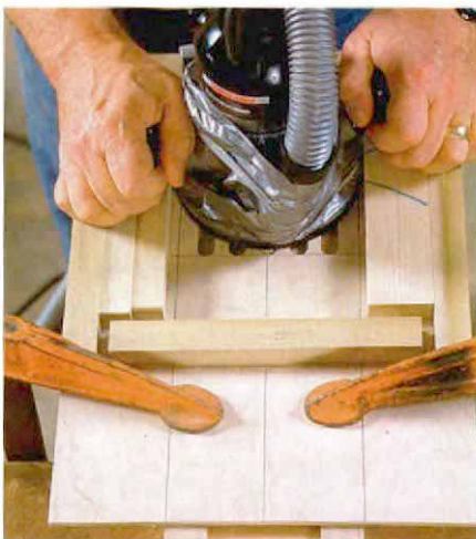
Move a block, make another cut. For each successive cut, one spacer block is moved to the other side of the jig. A vacuum keeps the jig clear of chips.
