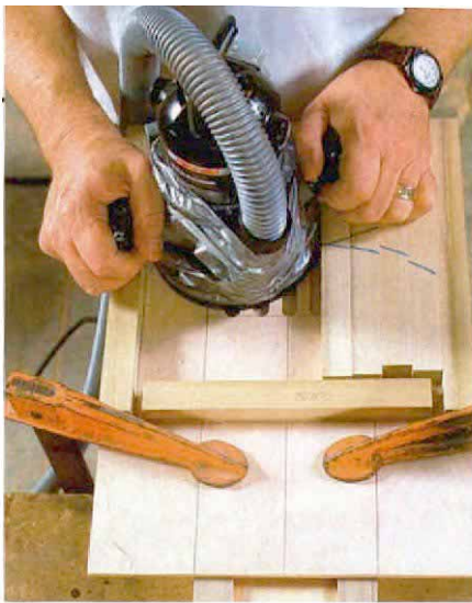
Spacers keep the router bit on track. The first plunge-router cut is made with the loose spacer blocks all to one side of the jig.
